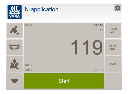
Initially the N-Sensor is in standby mode, i. e. it does not yet communicate to the spreader/sprayer and it does not yet log any data.
