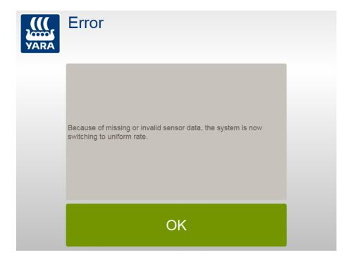
If the data from the N-Sensor is invalid or missing at all, the system automatically switches to uniform rate. Typically the reason for this warning is insufficient light for measurement or connection problems to the N-Sensor. More details can be found on the N-Sensor icon on the work screen (see section 4.1.2) and the diagnosis screen.
